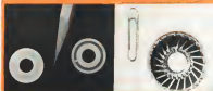
PRECISION polycrystalline element (left) has deposited tungsten, made by, and metal resistance film. Experimental transformer (right) consists of two 15-turn windings, magnetic film and dielectric, all deposited by vacuum evaporation process.
